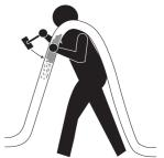
Start the pump for a few moments and make sure that the hose is free from "plugs"; the material comes out normally.
